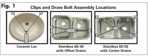
Depending on your sink type, the 3rd attachment point will be either the draw bolt assembly itself or another clip (see Fig. 1). If using another clip, you'll use both small holes to attach each end of the wire. Loop the wire underneath the clip holes to make a narrow "U" shape, leaving a 6 inch gap between the two sets of attached wires. If using the draw bolt assembly for the 3rd attachment point (See Fig. 5) mount the draw bolt assembly directly to the cabinet using the supplied screws.
